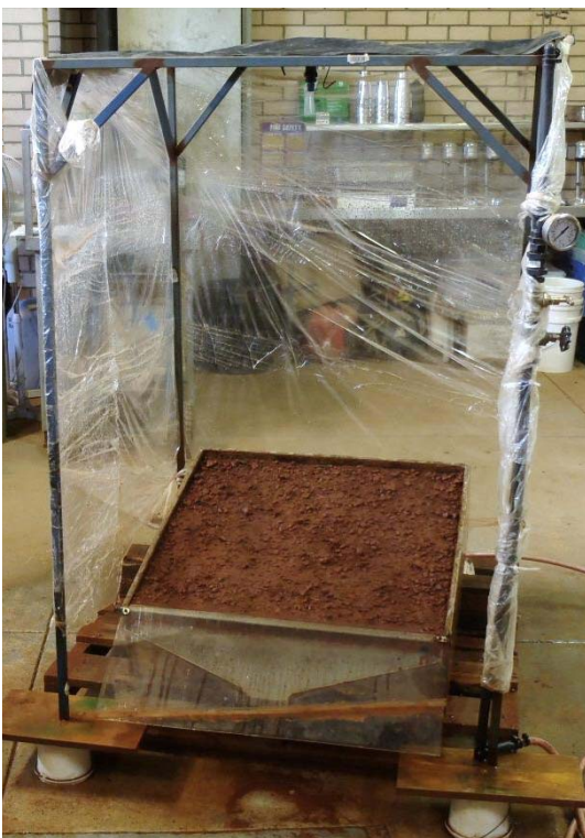
Plate 3.1: Laboratory scale rainfall simulator
